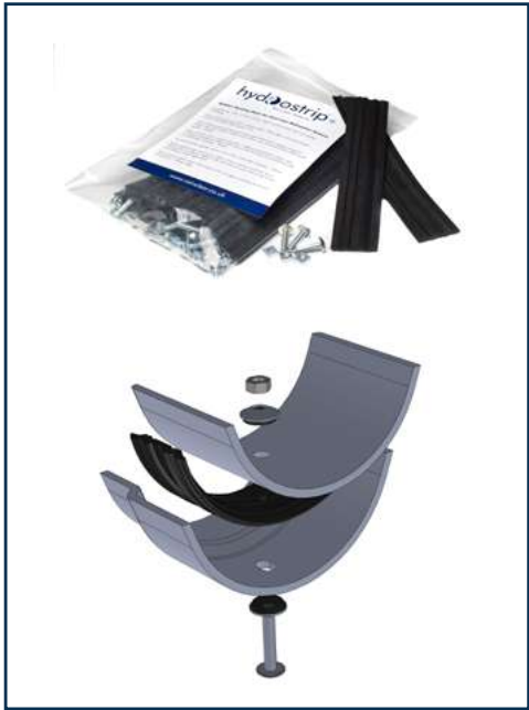
Fig 1. GSP: HYDROSTRIP GUTTER SEALING PACK (N.B. Not suitable for moulded or ogee profiles)
