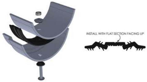
Fig 1. Illustration of how the specially designed & tested EPDM rubber strips seal the gutter lengths where they join.
