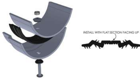
Fig 1. Illustration of how the specially designed & tested EPDM rubber strips seal the gutter lengths where they join.
