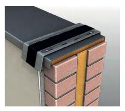
2. Position bracket with EPDM seal centrally over the wall. Maintain a minimum 10mm gap from the bracket inside return edge to the external wall surface finish. Illustration shows a render finish option which may be applied after installation of coping.
