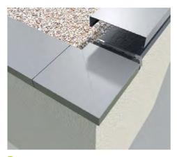
7. Starting at a corner working to your next junction, the last section of coping can be cut down on site to accommodate any variant dimensions between corner, pier and stop ends. Use touch up paint on cut edges. Contractor to use correct metal work tools, such as a circular saw.
