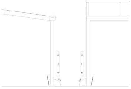
**Surface mounting**Mark outside edge of base platform position
