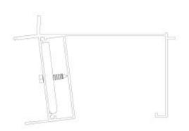
Fix the steel bar into position with drill screws no more than 20mm in length
