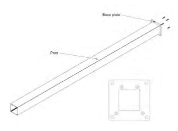
c) Fix standard base plates – if surface mounting with standard base plates or securing below ground.
