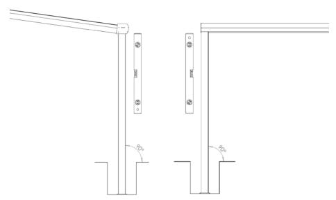
Once the roof beams are installed, check again that the veranda is installed at 90 degrees to the wall using a laser, or large set square. Then, using a spirit level check that the posts are vertical in both directions.
