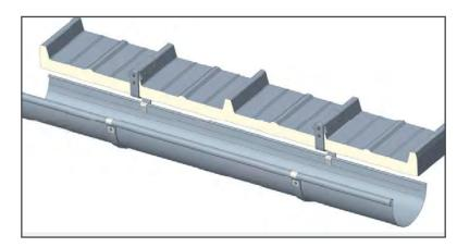
4. Hang the gutter and wrap the front part of the bracket over the beaded front edge of the gutter to secure it in place.
