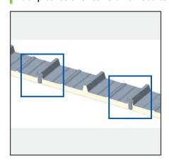
Place the clamp bracket with glued-in EPDM seal on every second roof panel ridge
