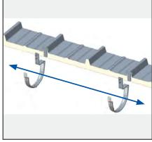
**Option a**) Installation without slope/fall: Align the gutter hooks in a position where there is a gap of approx. 2 mm between the lower cover shell of the sandwich panel and the gutter hook. Then properly fasten the gutter hooks at the front of the clamp to the speci ed holes in the clamp using two of the supplied self-drilling screws (RP-K, 6.3 x 25 mm).
