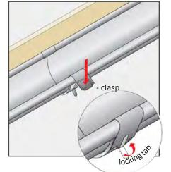
Locate the clasp over the front roll edge of the gutter. Pull union tight to the gutter and push the clasp down to squeeze shut.
