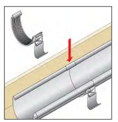
An EDPM rubber sealed union connector is used to connect the gutter lengths and angles together. Push open locking tab with thumb by pealing back rubber seal.
