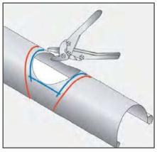
2. Use a hacksaw to make an initial hole in the gutter, and then use a set of tin snips to cut out the inner hole that you have marked out.
