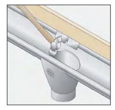
4. Tap the inner rough edges of the hole that was cut in the gutter, down into the outlet, to ensure a smooth flow of water.
