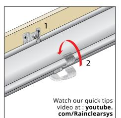
6. Locate the back of the fascia bracket over the rear edge of the gutter first, then pull the front of the fascia bracket up and over the front roll of the gutter. If you're finding this a bit of a struggle, use the bead connector (or other suitable tool) to open/raise the rear 'tab' of the fascia bracket a little.
