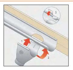
3. Attach the outlet to the gutter and fold the rear tabs of the outlet over the rear edge of the gutter, making sure the outlet is aligned correctly to accept the downpipe.
