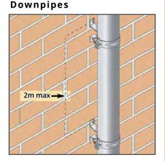
Downpipes should be installed using at least 2/no pipe clips per length. Mark out the clips locations and level with a sprit level or plumb line.
