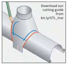
When installing a 'wrap around outlet' mark the desired location of the outlet by drawing a line either side of the outlet along its edge. Draw another line 20mm inside of the outer lines and join these inner lines together in an oval. This becomes the line to follow to cut out the hole.
