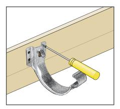
Generally position the fascia brackets at 915mm centres, using at least 3 brackets per gutter length. Use 2 screws on both the left and right fixing options (i.e. use 4 screws in total per bracket).
