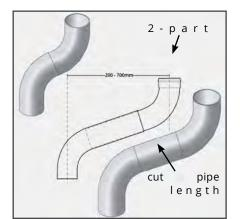
Offsets are achieved using either the 60mm fixed offset, 2no. 70° bends, the 2-part variable offset (for up to 700mm) or, for larger projections, by inserting a cut pipe length between the two bends.
