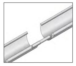
A bead connector (comes with the Union connector) is used to join two lengths of gutter. Insert the connector into the front roll of each gutter length. Allow for a 4mm expansion gap.
