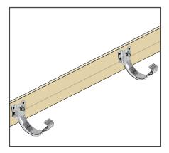
Use a string line to set out your fascia brackets along the gutter run allowing for a fall of 1:600 to 1:350 (max). (The system can be laid without a fall if you prefer)
