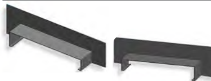
6. Ensure 31mm dimension is maintained from external wall surface finish to external face of coping. On deeper edged coping that exceeds the normal 75mm leg, it may be necessary to use a small self tapper on the coping return to secure it fully.
