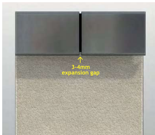
8. Maintain 3-4mm expansion gap at all joints.
