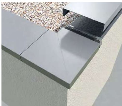
7. Starting at a corner working to your next junction, the last section of coping can be cut down on site to accommodate any variant dimensions between corner, pier and stop ends. Use touch up paint on cut edges. Contractor to use correct metal work tools, such as a circular saw.
