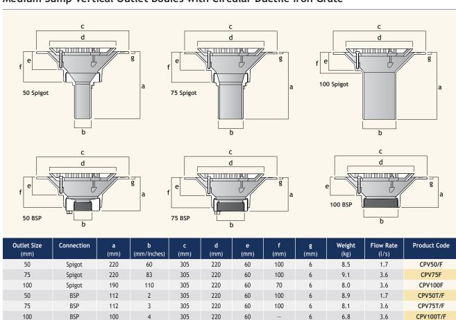
The Cast Iron Floor Drains include a clamping collar for a DPM or membrane to ensure a watertight seal. Available with either a BSP thread for connection to a Harmer threaded spigot adaptor and a spigot connection which can be connected direct to Harmer SML pipework to BS EN 877.
