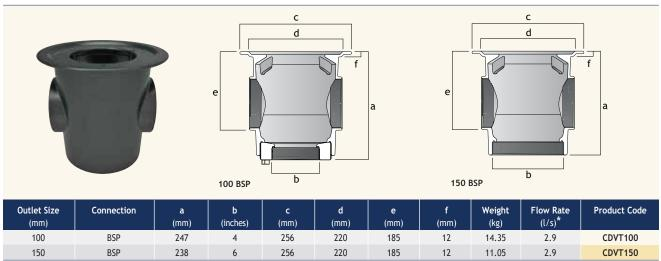
The flow rates relate to maximum sump capacity with use of compulsory clamp plate and 20mm head of water
