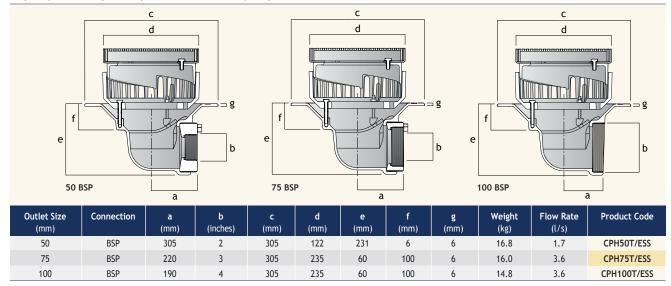
The Cast Iron Floor Drains include a clamping collar for a DPM or membrane to ensure a watertight seal. Available with either a BSP thread for connection to a Harmer threaded spigot adaptor and a spigot connection which can be connected direct to Harmer SML pipework to BS EN 877.
