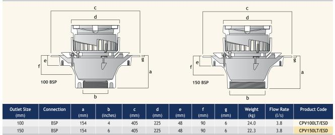
The Cast Iron Floor Drains include a clamping collar for a DPM or membrane to ensure a watertight seal. Available with either a BSP thread for connection to a Harmer threaded spigot adaptor and a spigot connection which can be connected direct to Harmer SML pipework to BS EN 877.
