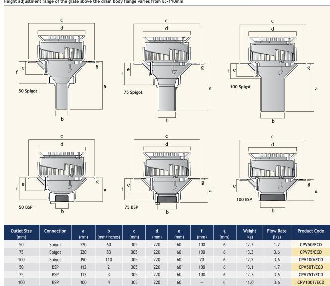
The Cast Iron Floor Drains include a clamping collar for a DPM or membrane to ensure a watertight seal. Available with either a BSP thread for connection to a Harmer threaded spigot adaptor and a spigot connection which can be connected direct to Harmer SML pipework to BS EN 877.
