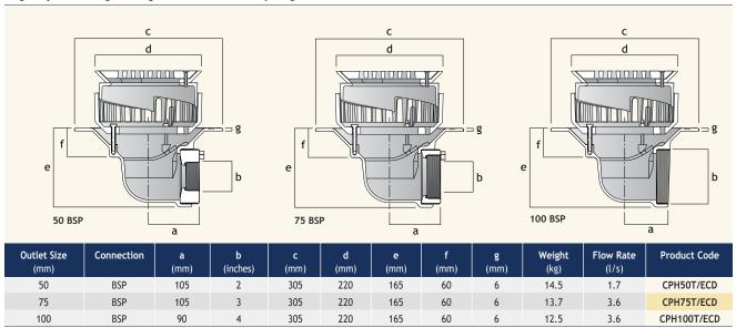
The Cast Iron Floor Drains include a clamping collar for a DPM or membrane to ensure a watertight seal. Available with either a BSP thread for connection to a Harmer threaded spigot adaptor and a spigot connection which can be connected direct to Harmer SML pipework to BS EN 877.
