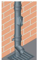
At ground level rainwater pipes can terminate with a shoe for free discharge over a gully or be directly connected into the gully.
