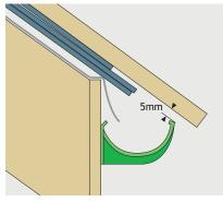
Using a straight edge or ruler, shim gutter brackets with 5mm clearance so that the last roof tile or slate will align with the mid point of the gutter.
