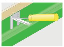
Fix gutters to fascia using combined top/back straps and No12 x 38mm round head wood screws and washers provided.
