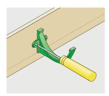
Generally, position brackets at 915mm centres. Allow at least 2 brackets per gutter length, 1 per angle and outlet.
