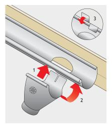
Attach the outlet to the gutter and fold the rear tabs of the outlet over the rear edge of the gutter, making sure the outlet is aligned correctly to accept the downpipe.
