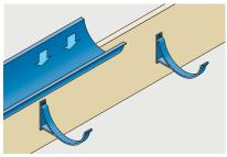
6. Clip gutter sections into brackets.
