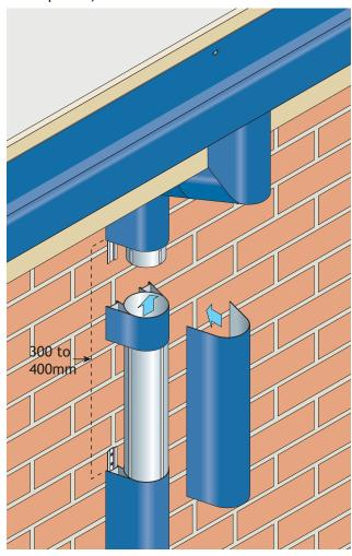
Build up and trim stack to within 300/400mm of underside of gutter and secure with fixing plates.  $\,$
