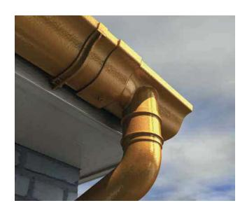
Heritage Victorian Ogee gutters are available in 3 sizes and 2 gutter lengths, together with a complete range of fittings. The traditional Ogee gutter profile is ideal for period applications and restoration. A left-hand socketed system, which can be finished to replicate cast iron or with BBA certificated powder coatings in a choice of colours.
