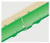
Finally, cone-off the exposed bolt stud and nut inside the gutter with a generous application of silicone sealant. Tool off excess silicone around the joint and from external surfaces.
