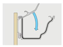
9. Compress joint union (back) and slide rear lock bar fully across joint.
