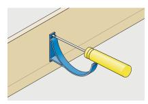
Generally position fascia brackets at 900mm centres in accordance with BS EN 12056-3:2000. Fix brackets with two No 12 x 38mm round-head screws.
