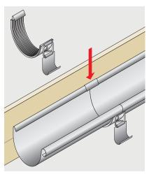
An EDPM rubber sealed union connector is used to connect the gutter lengths and angles together. Locate the union connector over the rear edge of the gutter.
