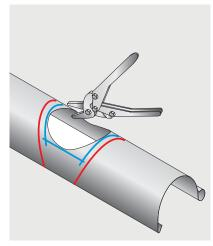
Use a hacksaw to make an initial hole in the gutter, and then use a set of tin snips to cut out the inner hole that you have marked out.
