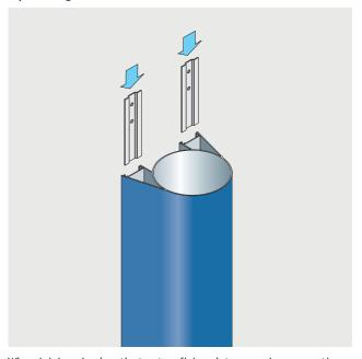
When joining pipe lengths tap two fixing plates per pipe connection into the pipe receiver rails using a block of wood to prevent damage.
