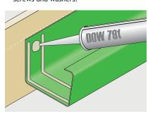
Thoroughly degrease all jointing surfaces and apply two 6mm beads of DOW 791 silicone sealant across back/sole/front surfaces.
