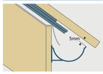
Using a straight edge or ruler, shim gutter brackets with 5mm clearance so that the last roof tile or slate will align with the mid point of the gutter.
