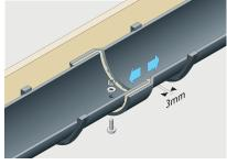
Insert the spigot end of the gutter allowing a 3mm expansion gap. Secure joint using bright zinc plated, mild steel M6 x 25mm nut, bolt and washer provided. (Bolt head preferably to underside).
