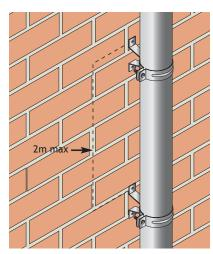
6. Downpipes should be installed using at least 2/no pipe clips per length. Mark out the clips locations and level with a sprit level or plumb line. Open the tightening screw to allow the pipe to be inserted, close the clip and re-tighten, making sure not to over tighten and damage the downpipe.
