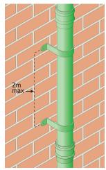
Where uneared pipework is being used it must be secured at maximum 2m centres.
