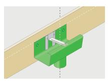
Plumb line outlet positions with gullies at ground level and mark fixing positions. Pilot 3.5mm diameter holes and loosely fit using No12 x 38mm round head wood screws and washers.
