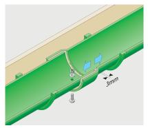
Insert the spigot end of the gutter allowing a 3mm expansion gap. Secure joint using aluminium M6 x 20mm nut, bolt and washer provided. (Bolt head preferably to underside).
