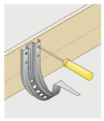
Generally position the fascia brackets at 915mm centres, using at least 3 brackets per gutter length. Use 2 screws on both the left and right fixing options and 1/no underneath the gutter securing tab.
