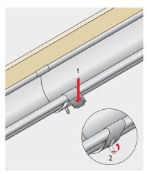
Locate the clasp over the front roll edge of the gutter. Push down on top of the clasp and squeeze the clasp shut. Fold the locking tab over to fully secure.
