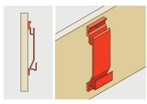
Bracket for Half Round and Deep Run gutters (Supplied to colour match gutter)
