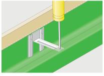
Screw the front end of the top straps to the preformed holes in the top lip of the gutter. Use the pan head fixing screw provided.
