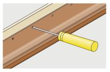
Fix all components and gutter lengths direct to the fascia with a single roundhead screw through the back edge at 900mm centres. Drill 8mm holes 18mm from the top edge.
