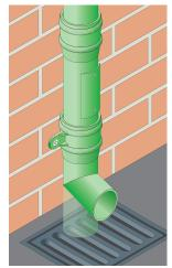
At ground level rainwater pipes can terminate with a shoe for free discharge over a gully or be directly connected into the gully. In the case of direct connections it is recommended that an access pipe fitting is included within 750mm of ground level.
