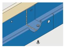
Secure joints with aluminium M6 x 12mm nuts, bolts and washers provided taking care not to over tighten or displace sealant from within the joint.
