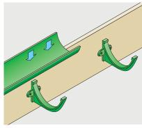
Lower the gutter onto the brackets ensuring sufficient clearance for the gutter joint. Clip gutter into bracket.
