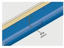
4. Line and level gutter lengths allowing for 4mm expansion gaps at joints.
