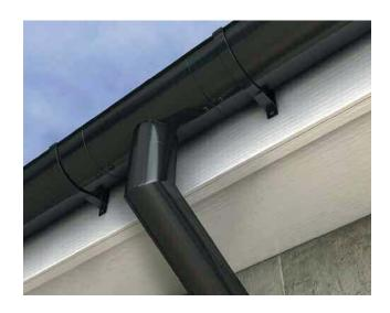
AX Beaded Deep Run Gutters combine economy and efficiency where a high capacity gutter and extra performance is required. Available in one size and in standard 3m gutter lengths, together with a complete range of fittings. Factory finished in a choice of BBA approved polyester powder coatings.
