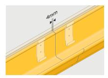
6. Check and reset 4mm expansion gap as necessary.
