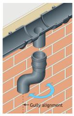
Where square or rectangular pipes are being installed and offsets are required, alignment between the gutter outlet and gully must be exact.
