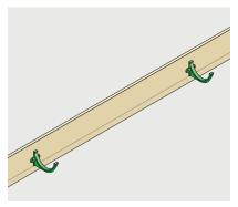
Use a string line to set out brackets to a fall of 1:600 to 1:350 (max) or if not possible, level.
