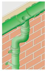
Commence installation from the gutter outlet by fitting and adjusting the one part or two part offsets.
