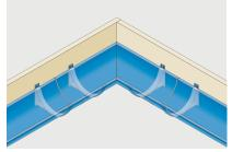
Offer angle pieces and outlets to the fascia. Lower gutter sections onto the brackets leaving a 4mm expansion gap between gutter sections and allow sufficient clearance for the gutter joint.
