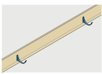
Use a string or laser to establish a true line and level of the gutter. Prepare to use packing pieces under brackets where there are depressions.
