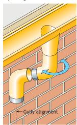
Check alignment of gutter outlet to gully. Where square or rectangular pipes are being installed and offsets are required, alignment between the gutter outlet and gully must be exact.
