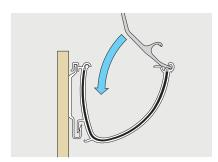
Compress joint union and start lock bar across joint.
