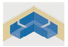
Position angles, mark fixing positions and pilot 3.5mm diameter holes, fit top strap and loosely fix using No12 x 38mm roundhead screws.
