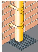
Where rainwater pipes directly connect to the gully it is recommended that an access pipe is fitted no more than 750mm above ground level.
