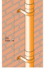
Pipe clips support and hold the rainwater pipe to the structure. All three types of pipe clip, Standard, Small Base and Extended Base can be used.
