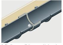
Finally, cone-off the exposed bolt stud and nut inside the gutter with a generous application of silicone sealant. Tool off excess silicone around the joint and from external surfaces.
