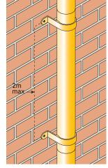
Pipe clips support and hold the rainwater pipe to the structure. All three types of pipe clip, Standard, Small Base and Extended Base can be used to conceal the pipe joints.
