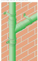
Bends and branches are secured into the pipe socket. Where additional fixing is required e.g a change of direction at a bend, use additional pipe clips.
