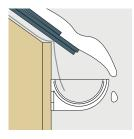
Fix brackets so as to position the gutter centrally and as close below the roof edge as possible, taking into consideration locality and roof slope finish.
