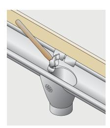
Tap the inner rough edges of the hole that was cut in the gutter, down into the outlet, to ensure a smooth flow of water.
