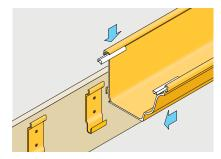
2. Position gutters loosely, do not lock down.
