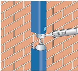
Pipe lengths are connected by sliding new pipe sections down over the fixing plates of the pipe below.
