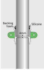
Allow a 4mm expansion gap between pipe end and socket, and insert a 6mm backing foam into the pipe joint. Seal with DOW 791 silicone sealant.
