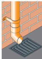
At ground level if the rainwater pipe does not connect directly to the gully, pipes can terminate with a shoe fitting for free discharge over the gully.
