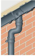
Commence installation from the gutter outlet by fitting offsets.
