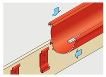
2. Position gutters loosely, do not lock down.
