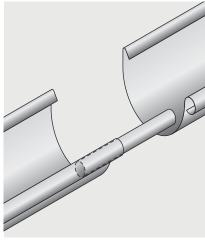
3. A bead connector is used to join two lengths of gutter. Insert the connector into the front roll of each gutter length. Allow for a 4mm expansion gap.
