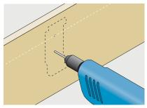
2. Position and pilot 3.5mm diameter hole.
