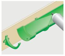
Cast gutters overlap at the joint with a spigot and socket. Thoroughly clean and degrease the ends that must be jointed.
