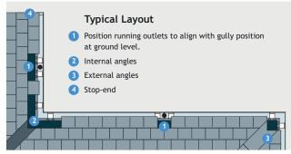
After setting out angles and outlets, fit gutters and brackets according to installation procedures for the specific rainwater system being used, as detailed in this brochure.
