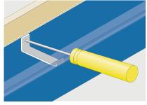
Align gutter lengths correctly for final positioning. Engage top straps and fix back securely to fascia.
