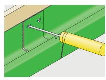
Slide in union joints and back fix to fascia board using No12 x 38mm round head wood screws and washers. Slide in next gutter and repeat process.
