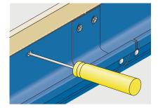
Tighten all fascia fixing screws and fit top straps if required otherwise screw back securely to the fascia using No12 x 38mm round head wood screws and washers provided.
