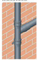
Bends and branches are secured into the pipe socket.
