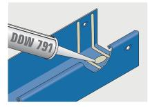
Thoroughly degrease all jointing surfaces and apply two 6mm beads of DOW 791 silicone sealant either side of and around the slotted fixing holes.
