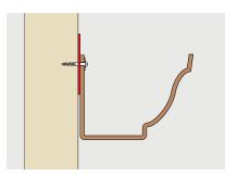
Note any uneven surfaces on the fascia and make adjustments if possible. Where shallow depressions occur, packing pieces can be used under gutter lengths.
