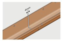
When joining gutter lengths, allow for a 4mm expansion gap.
