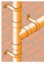
Continue to assemble the stack taking care not to scratch the pipe coating whilst sliding pipe clips into position.
