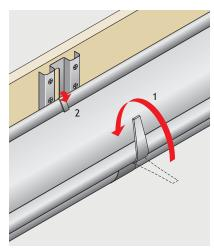
6. Locate the gutter into the fascia bracket and seat level, then fold the front tab of the fascia bracket around the front roll and into the gutter. Fold the rear tab of the fascia bracket down and over the rear edge of the gutter.
