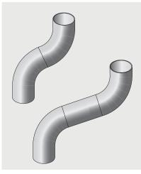
5. Offsets are achieved using 2/no 70° bends, with larger offsets being made by inserting a pipe length between the two bends.
