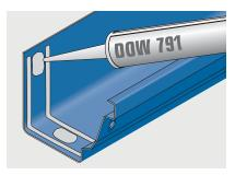
Thoroughly degrease all jointing surfaces and apply two 6mm beads of DOW 791 silicone sealant either side of and around the slotted fixing holes to inside back/sole/front surfaces.
