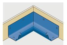
Position angles, mark fixing positions and pilot 3.5mm diameter holes and loosely fit using No12 x 38mm round head wood screws and washers provided.
