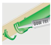
Apply two 6mm beads of DOW 791 silicone sealant either side of, and around the fixing hole.
