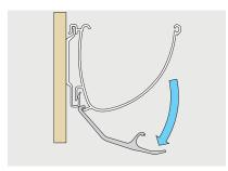
4. Lock down gutter with Aqualine jointing tool.
