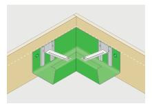
Position angles, mark fixing positions and pilot 3.5mm diameter holes. Loosely fit using No12 x 38mm round head wood screws and washers provided.
