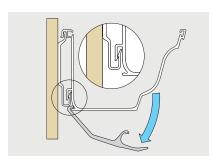
4. Lock down gutter with Aqualine jointing tool and check for full location.
