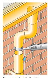
Commence installation from the gutter outlet by fitting and adjusting the two part offsets. Check vertical plumb line and assemble internal spigot joints using DOW 791 silicone sealant then fit first pipe clip.
