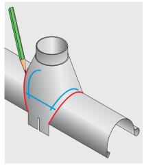
When installing a 'wrap around outlet' mark the desired location of the outlet by drawing a line either side of the outlet along its edge. Draw a further line 20mm inside of the outer lines and join these inner lines together in an oval pattern. This becomes the marking for the cut out hole.
