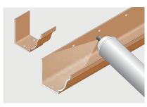
De-grease and clean each union and gutter length/fitting to a distance of 50mm - 100mm from the end.
