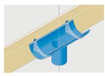
4. Plumb line outlet positions with gullies at ground level.
