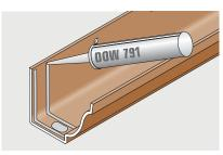
Apply two 6mm beads of Dow Corning 791 low-modulus Type A silicone sealant either side of, and around the fixing holes. Silicone sealant must be applied only to completely dry surfaces.
