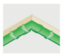
Plumb line outlets with gullies at ground level. Position angles, allowing an additional bracket adjacent to the joint with the gutter length.
