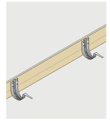
2. Use a string line to set out your fascia brackets along the gutter run allowing for a fall of 1:600 to 1:350 (max).
