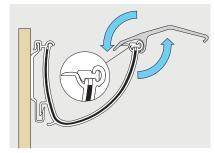
11. Reverse tool apply **equal** pressure around **pivot** point to complete lock bar positioning fully across joint. Take care not to dislodge gutter from fascia
