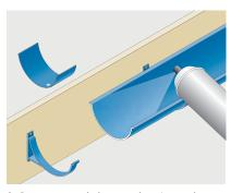
8. De-grease and clean each union and gutter length/fitting to a distance of 50 - 100mm from the end.
