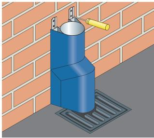
Commence installation by fitting fixing plates to the drain connector component and then fixing to the wall.
