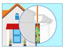
**5.** For a downpipe that has been blocked (by debris flushed down through the outlet from the gutter), buy a drainage rod, available from most hardware shops, then push through from above and out of the gutter shoe at the bottom.
