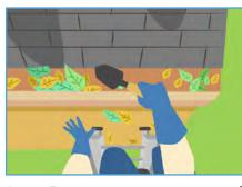
3. Ensure gutters and downspouts are clear and free from any blockage. Using gloved hands or a gutter scoop, remove any leaves and debris from the gutters and drop them in a bag or bucket that you can easily carry down the ladder and get rid of appropriately afterwards.
