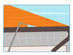
**9. If pressure washing, the head of the water lance** should be kept at least 500mm away from the surface at all times, and the pressure should be restricted to less than 1500psi.
