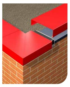
Start at a corner working to your next junction. The last section of coping can be cut down on site to accommodate any variant dimensions between corner, pier and stop ends. Use touch-up paint on cut edges. When cutting, make sure to use the correct metalwork tools to obtain a clean cut and dress any sharp burr edges.
