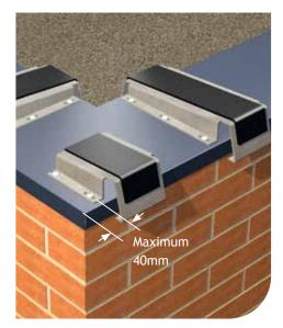
5. Always secure additional half brackets for corners and piers — the first fixing point with a maximum of 40mm from the external wall finish.
