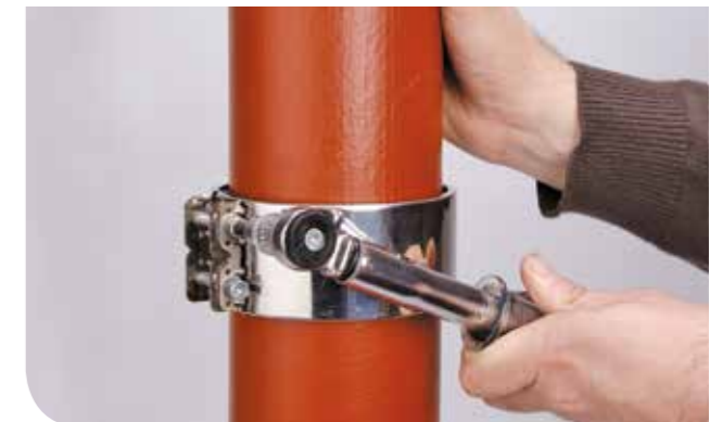
4. Evenly tighten the bolts to the required torque setting. The coupling should only be tightened once, because it cannot be dismantled and re-used. (See Couplings Data page 55)
