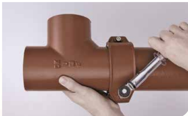
5. Check the alignment of the assembly before tightening the bolts. Alternately, tighten the bolts to ensure that the coupling is aligned evenly. Bolts should be tightened until a reasonable resistance is achieved - recommended torque setting 22 Nm.
