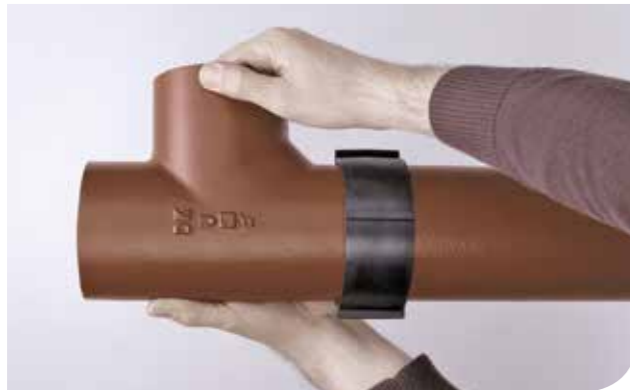
3. Ease the next pipe or fitting into the EPDM rubber gasket making sure that the spigot end is against the central inner register.
