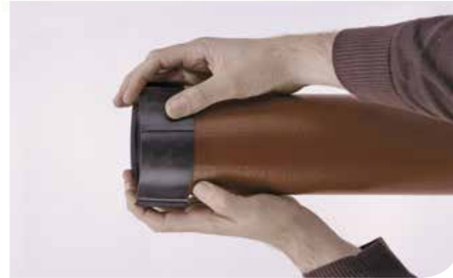
2. Push the EPDM rubber gasket over the end of the pipe or fitting, ensuring that the central inner register is abutted against the spigot end.
