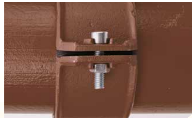
6. All Ductile Iron couplings use an M8 bolt and require a 6mm allen key. The coupling incorporates an anti-turn feature which holds the bolt nut in place without the need for a secondary tool. (See page 47 and 59 for details of fixing tools)
