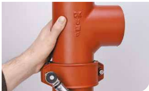
5. Check the alignment of the assembly before tightening the bolts. Alternately, tighten the bolts to ensure that the coupling is aligned evenly. Bolts should be tightened until a reasonable resistance is achieved - recommended torque setting 20 Nm.
