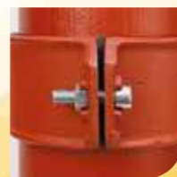
6. For electrical continuity, hand-tighten the electrical continuity screws on both sides. Ensure screws pierce external coating of pipe when tightened. (See page 55)
