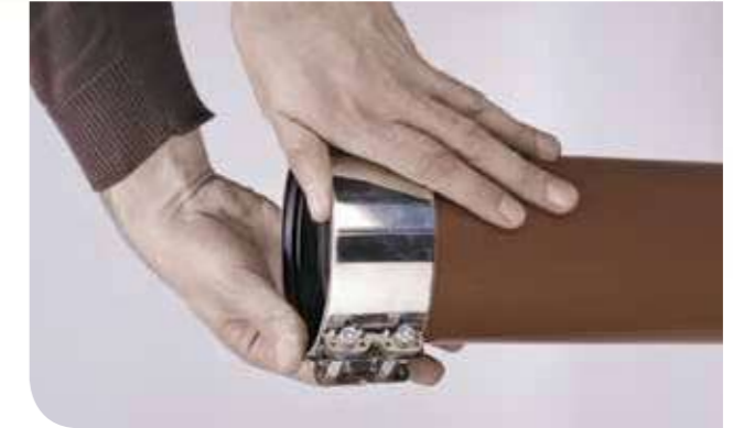
2. Ease-in one side (next to the continuity spur) then push on the opposite side of the coupling to fully seat, ensuring that the central inner register is abutted against the spigot end.
