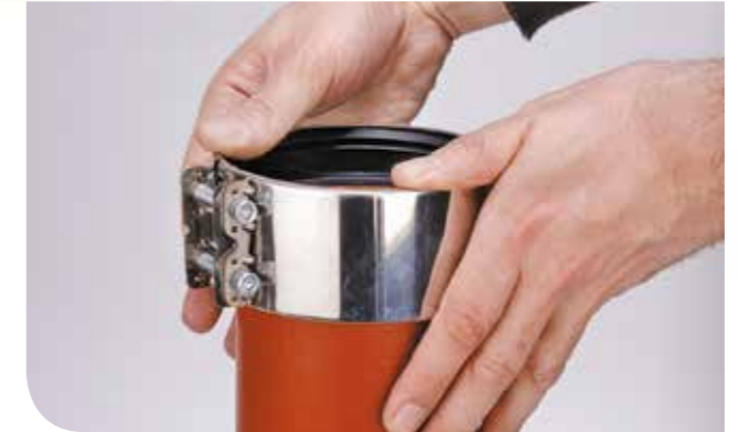
2. Ease-in one side (next to the continuity spur) then push down on the opposite side of the coupling to fully seat, ensuring that the central inner register is abutted against the spigot end.
