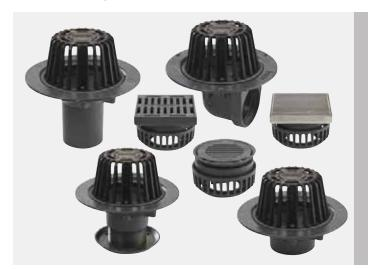
The Harmer cast iron medium sump range is a compact outlet body in vertical and horizontal variations for connection to 50, 75 and 100mm pipe work. Vertical bodies come with either spigot or threaded outlets and horizontal body versions are available in threaded only.
