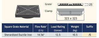
\*For 100mm outlet size, maximum pipe capacity to BS EN 12056 applies.
