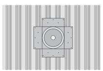
Plan view of Harmer outlet body in the Metal Deck Support Plate fixed to the structural metal deck.
