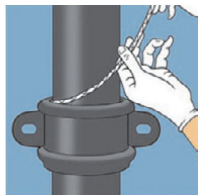
1. Centrally align the pipe spigot within the socket and wet the cord.
