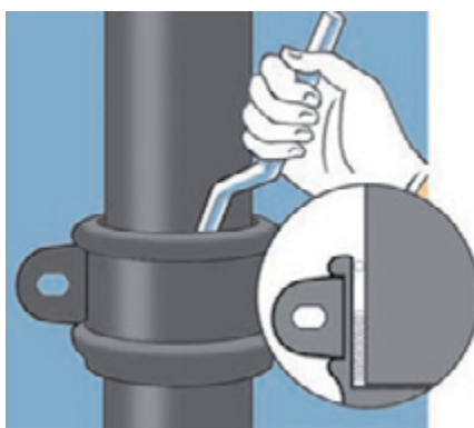
2. Caulk this into the socket, up to 30mm from the top. This will centralise the pipes and provide a backing for the top 30mm of the joint.
