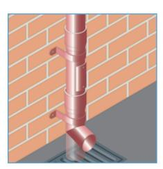
At ground level, rainwater pipes can terminate with a shoe for free discharge over a gully or be directly connected into the drainage system.
