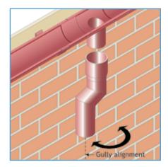
1. SnapIT pipes have an integral swaged end to allow ease of connection.
