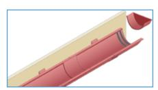
Running outlets and angles can be jointed using the same union clip method as described in Fig.4-7. Stop ends are internally fixed in left or right hand position using the same method but without the union.
