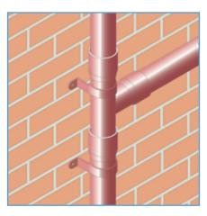
5. Bends and branches are secured into the swaged pipe end.
