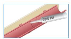
Seal both edges of the union with low modus silicone sealant DOW791, removing any excess. All cut edges must be re-coated using Touch-up paint (available in 250ml tins).
