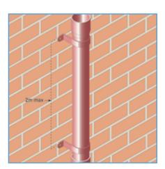
A pipe clip should be fixed directly underneath the pipe swage with additional clips at 2m maximum intervals. Clips to be fixed with plastic wall plugs & No12 x 2" roundhead screws SCREW20 (dependant on substrate)
