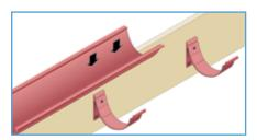
3. Locate gutters into the brackets and allow 4mm expansion gap. Clip the gutters into position making sure that the gutter is securely fixed into the bracket.
