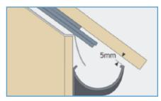
Using a straight edge or ruler, shim gutter rackets with 5mm clearance so that the last roof tile or slate will align with the mid point of the gutter.
