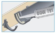
Apply two 6mm beads of DOW 791 silicone sealant either side of, and around the fixing hole.
