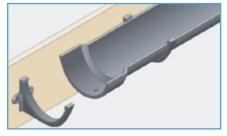
Cast gutters overlap at the joint with a spigot and socket. Thoroughly clean and degrease the ends that must be jointed.
