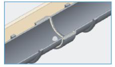
Finally, cone-off the exposed bolt stud and nut inside the gutter with a generous application of silicone sealant. Tool off excess silicone around the joint and from external surfaces.
