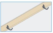
3. Use a string line to set out brackets to a fall of 1:600 to 1:350 (max) or if not possible, level.
