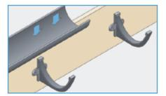
5. Lower the gutter onto the brackets ensuring sufficient clearance for the gutter joint. Clip gutter into bracket.
