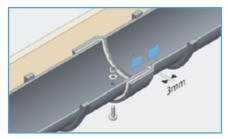
Insert the spigot end of the gutter allowing a 3mm expansion gap. Secure joint using bright zinc plated, mild steel M6 x 25mm nut, bolt and washer provided. (Bolt head preferably to underside).
