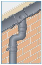
Commence installation from the gutter outlet by fitting offsets. vertical plumb line Check positioning and seal spigot and socket joints using DOW 791 silicone sealant.
