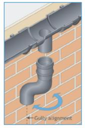
Where square or rectangular pipes are being installed and offsets are required, alignment between the gutter outlet and gully must be exact.
