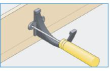
2. Generally, position brackets at 915mm centres allowing additional brackets either side of where gutter joints will occur.
